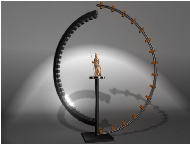
Figure 11: An Evolved Light Stage includes a stationary array of cameras, seen at right, that record the artifact from a one-dimensional array of directions, and a motorized platform that can rotate the artifact a set number of degrees for every rotation of the light stage arm. The device would capture a complete light field of the artifact for every direction of incident illumination, allowing artifacts to be rendered from any viewpoint as well as illuminated from any direction.
